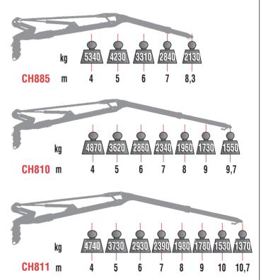
Actual lifting capacity depends on which link, rotator and harvester head is used.
