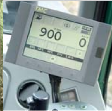
The software feature that optimises the engine's RPMs helps to lower fuel consumption and reduce noise levels. The new Eco III forwarders help machine operators to run their machines even more economically than before.
